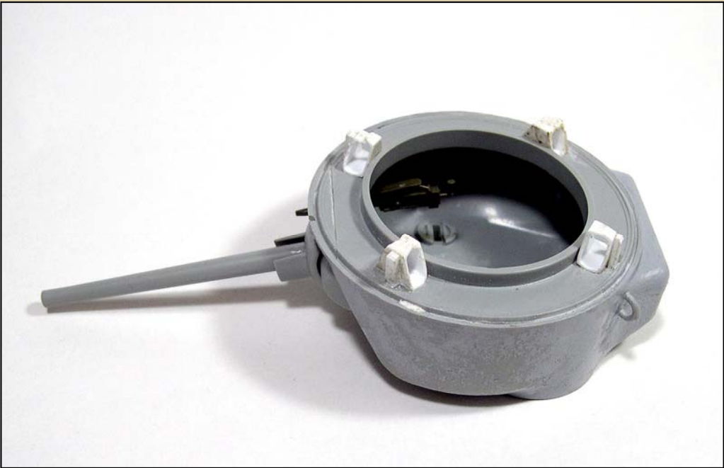
Above. The spacers I added to adapt the turret to the larger Asuka turret ring.
