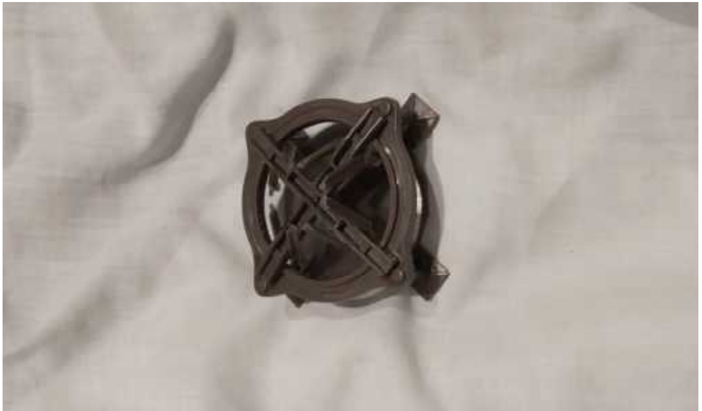
This is the 3 part Base piece (The MobileLaunch Pad) assembled and ready to prime. I will use Mr Finishing Surfacer 1500 Black as it gives a beautiful smooth coat and thins readily with Mr Levelling Thinner.
