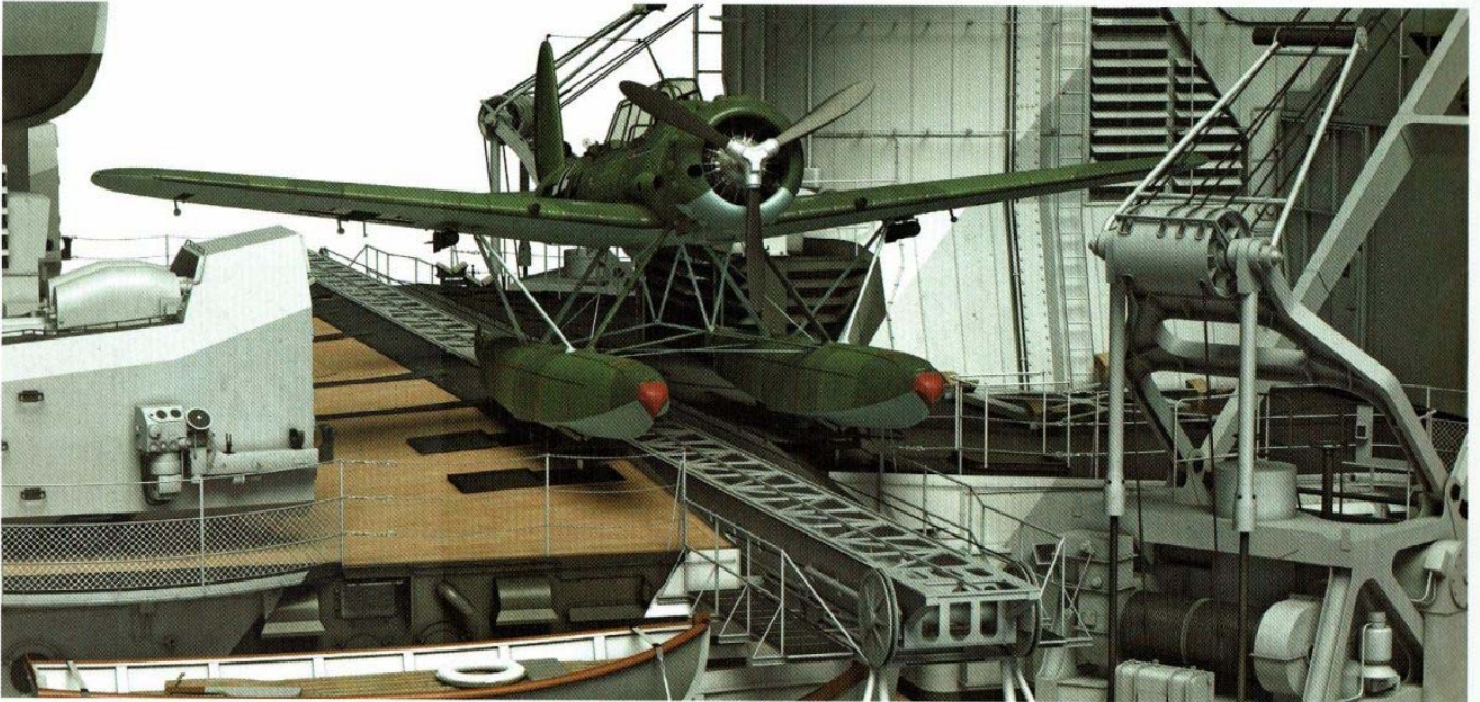
Floatplane in a stand-by position – sitting on retractable aircraft cradle. Wings have been unfolded for takeoff.
