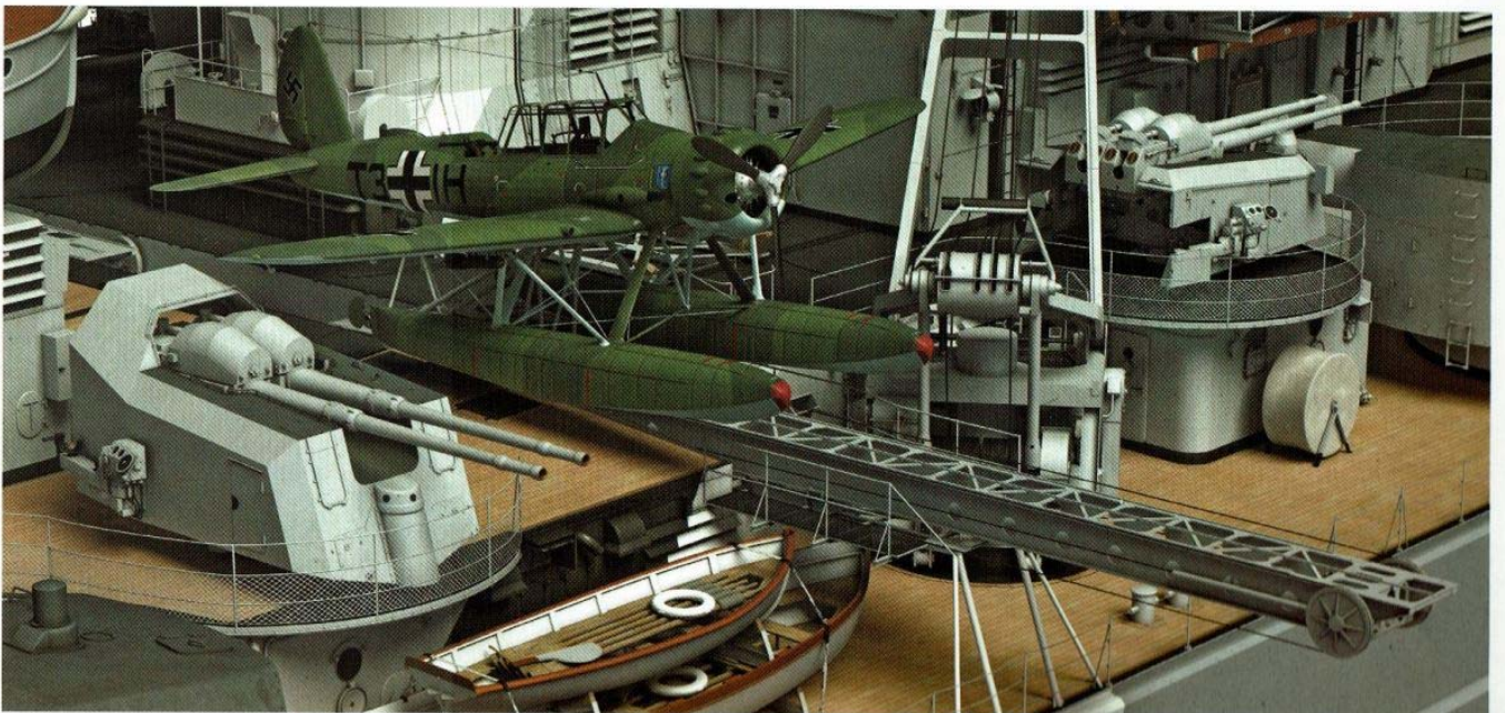
Floatplane in a stand-by position – sitting on retractable aircraft cradle. Wings have been unfolded for takeoff.
