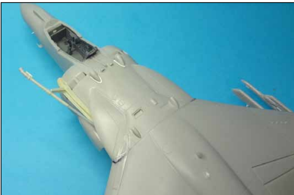
12 Upper view showing refuelling probe, new GPS 'brick' from styrene at rear of the jet and the repositioned fire extinguisher inlets ('frogs eyes') behind the cockpit with the new mounts from styrene. These had to be moved outboard to allow the canopy to open.
