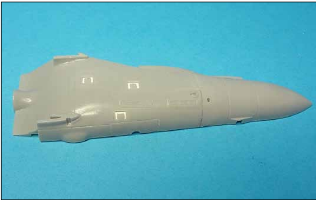
07 Exterior shot giving good view of the 3 step openings.
