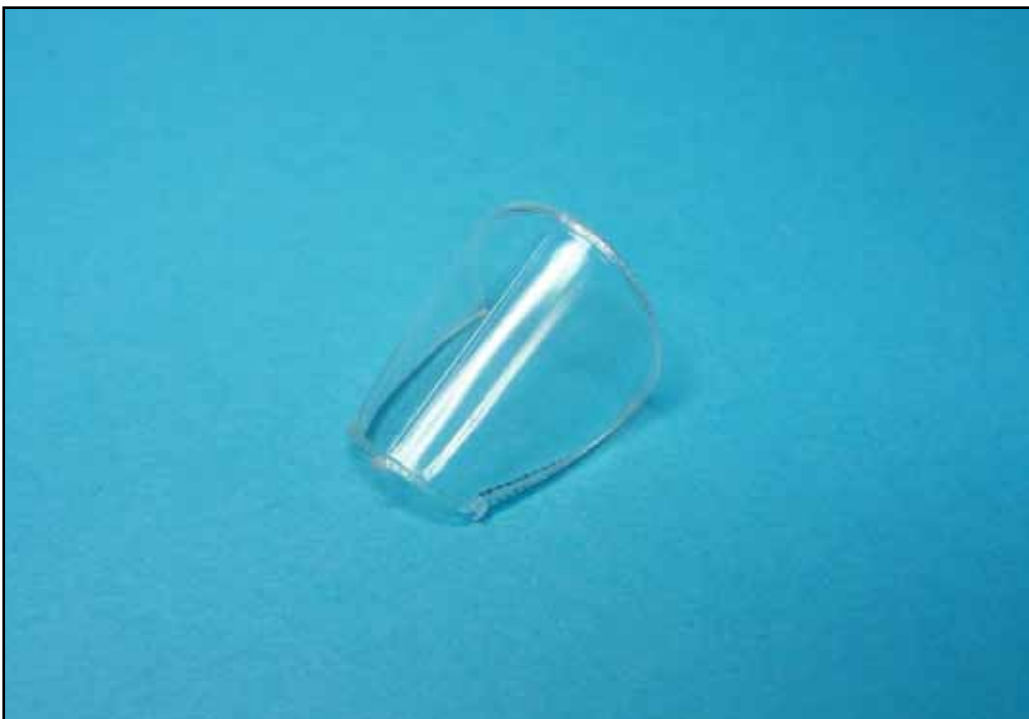
18 Windscreen as supplied in the kit with a mould seam down the middle. This seam allows the canopies to have their bubble cross section, but need to be removed from the finished parts.
