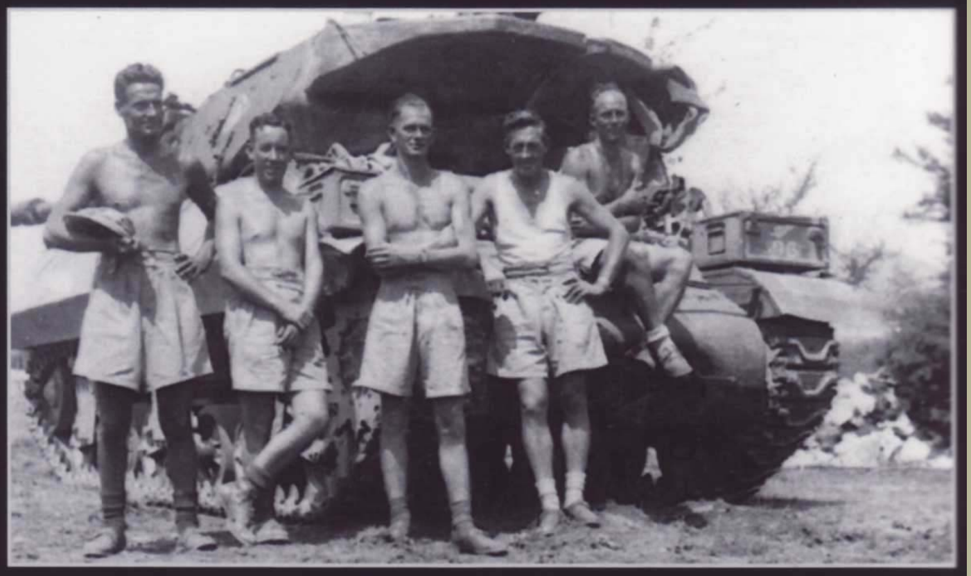
A Kiwi Achilles in Italy. Note what appears to be T54E1 type tracks, and the usual Kiwi additions of spare ammo boxes mounted to the front fenders. (via Armour Camouflage & Markings of the 2nd New Zealand Division by Jeffrey Plowman).
