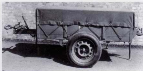
1-ton trailers were built in limited numbers during the war but did meet with greater demand in the post-war years. This image shows a Dashwood-built No. 5 Mk 1 trailer. It is a late model with smaller 900 x 13 tyres and a large castor wheel on the front jockey leg.
