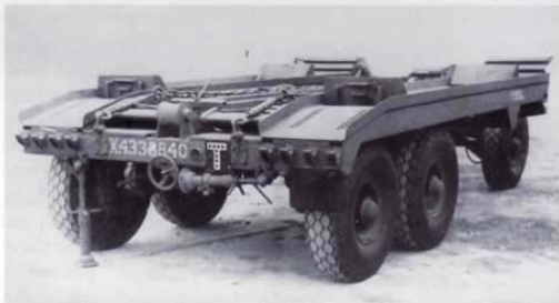
The Crane 7.5-ton Light Recovery Trailer issued to LADs. A manually operated winch with 50 feet of cable could be used when the prime mover had no winch. Reversible ramps (one side smooth and the other ribbed) allowed the loading of both tracked and wheeled vehicles. These were stowed between the body channels when not in use.
