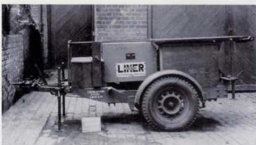
A number of 10cwt lightweight chassis were used for specific roles, including this Liner portable saw bench.
