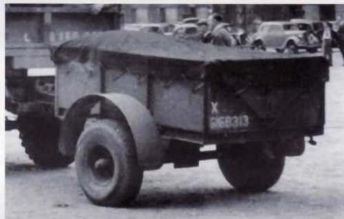
1-ton trailers were built in limited numbers during the war but did meet with greater demand in the post-war years. This image shows a Dashwood-built No. 5 Mk 1 trailer. It is a late model with smaller 900 x 13 tyres and a large castor wheel on the front jockey leg.
