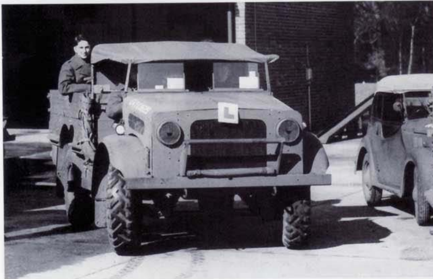
Shown just before issue to the military, the early MWD models were supplied without a body tilt. Clips to hold the crew's rifles are clearly observed in the cab area. Weapons must have been in short supply at the time, as one is a wooden dummy. Note the body sides were hinged just above the rear-wheel arch.
