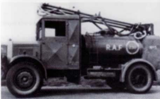
The triple-boom Refueller. The vehicle would have been parked in a central position to allow three fighter aircraft to be refuelled at the same time.
