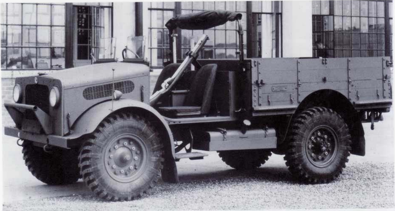
Shown just before issue to the military, the early MWD models were supplied without a body tilt. Clips to hold the crew's rifles are clearly observed in the cab area. Weapons must have been in short supply at the time, as one is a wooden dummy. Note the body sides were hinged just above the rear-wheel arch.
