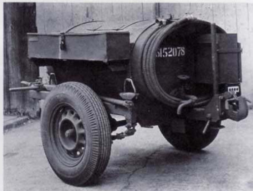
A lightweight 100-gallon Water Tank, again with the rear tow hitch and stowage boxes for hoses and filters.
