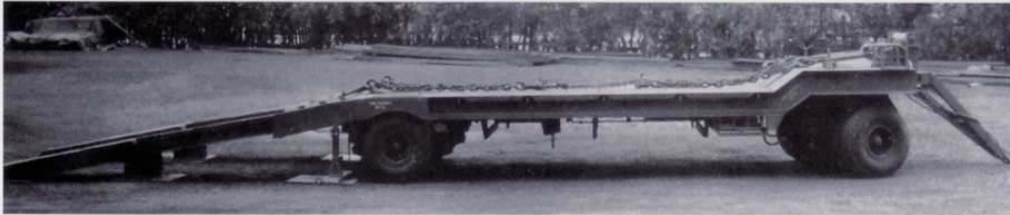
The Multiwheeler/SMT low-loading drop-frame trailer of 20-ton capacity was built from rolled-steel sections. The trailers could, if required, handle tanks weighing up to 20 tons, but their main role was the transportation of heavy construction equipment. The 16 wheels were shod with 29 x 8 HD tyres.
