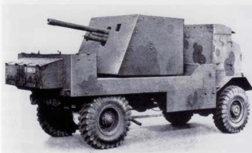
One hundred and seventy five 6 pdr anti tank Deacons were produced on the Matador chassis and all were issued for service in the Middle East and served until the end of 1943. The gun was mounted in a turret mounted in the centre of the body with a 319 degree traverse, a small number were sold to the Turkish army from stocks held in 1944.
