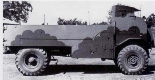
From redundant stocks held in 1943 a number of Deacons were converted to armoured ammunition carriers at the AEC factory and were issued in the main to anti tank batteries.
