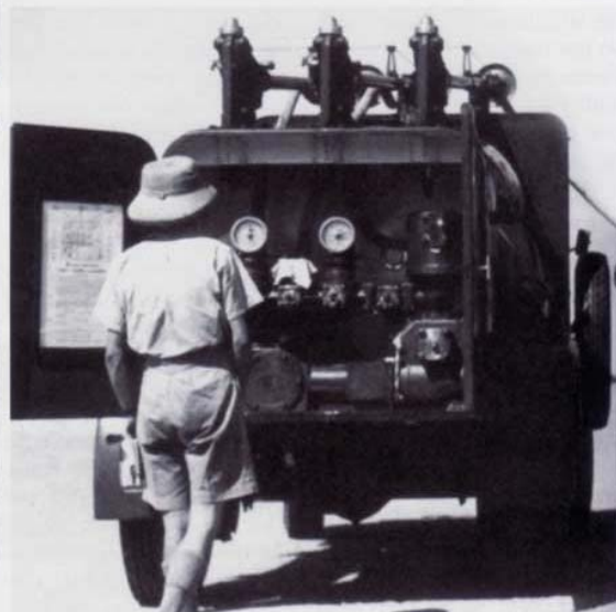
The pump and filters on a triple-boom Refueller. The equipment was supplied by Zwickey.
