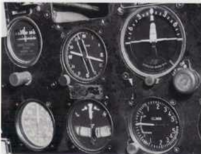
(Above) As noted, there were few changes to the main instrument board during production of the Dash-1 family, but numerous changes above, below, and around the panel. This FG-1A (BuNo 76510) has most of its armament switches moved to the eyebrows, a rocket control panel to the right, and a flare pistol cartridge box below. Arrows mark the chart board rails - the chart board was part of each pilot's navigational equipment, carried to the plane before flight. Since the Navy's chart boards came in several sizes, the Corsair's chart board rails were adjustable to hold the different boards in position.
