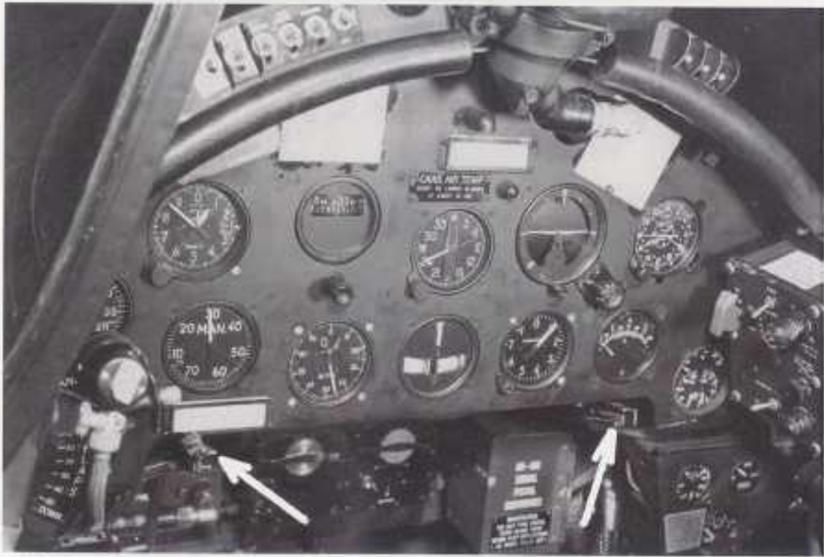
(Above) As noted, there were few changes to the main instrument board during production of the Dash-1 family, but numerous changes above, below, and around the panel. This FG-1A (BuNo 76510) has most of its armament switches moved to the eyebrows, a rocket control panel to the right, and a flare pistol cartridge box below. Arrows mark the chart board rails - the chart board was part of each pilot's navigational equipment, carried to the plane before flight. Since the Navy's chart boards came in several sizes, the Corsair's chart board rails were adjustable to hold the different boards in position.
