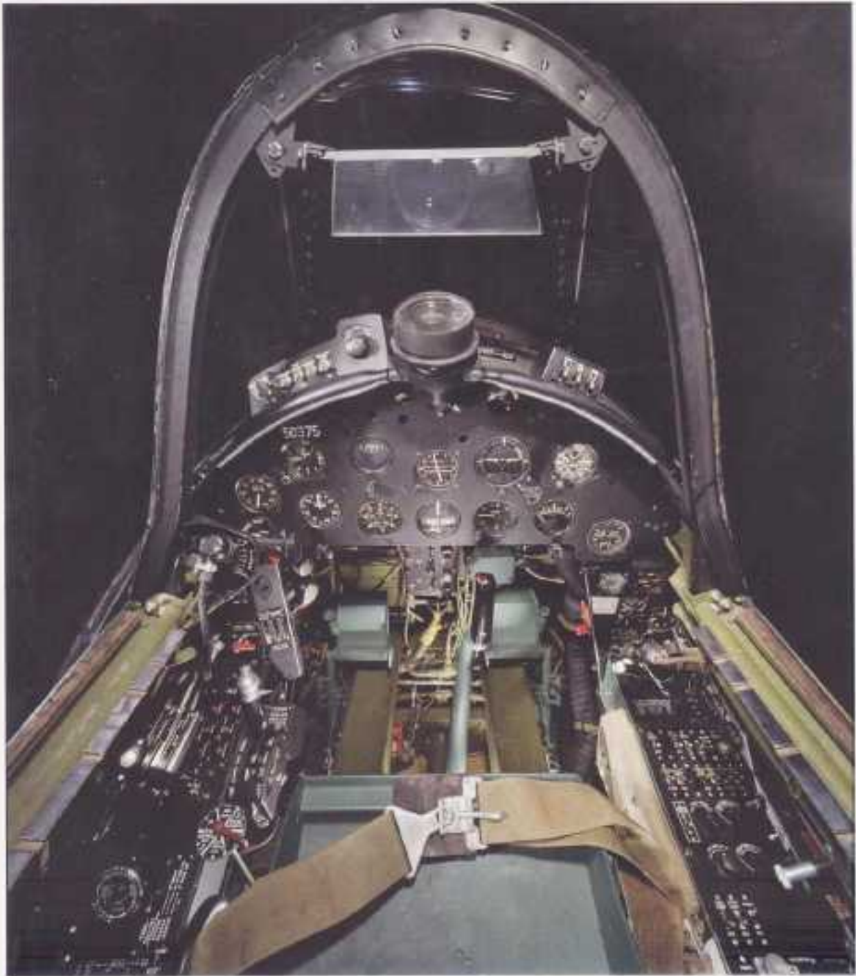
The National Air and Space Museum's F4U-1D (BuNo 50375) was Fought's 2815 th Corsair and the 26 th -1D built. Most cockpit features had been introduced on the F4U-1A, with updates to manage the -1D's fuel, arm, and radio revisions. The cockpit paint is generally Interior Green (approximately 34151 or FS5956), with subassemblies such as the seat, joy stick, and rudder pedals finished in the same Dull Dark Green (a touch darker than 34092) paint first used on the Birdcage Corsair. Most of the instrument panels are Instrument Black, with smaller placards in unpainted black plastic. Note the gunsight mirrored in the rectangular reflector atop the windshield's armored glass panel. (NASM)
