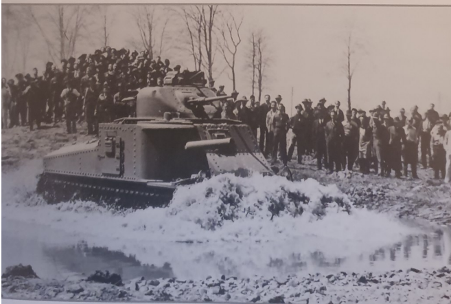
Above: The first production pilot M3 completed by Chrysler splashes through a pond during a demonstration of its fording capabilities during the rollout on 24 April 1941. The Medium Tank M3 had a maximum fording depth of 40 inches. Military History Institute
