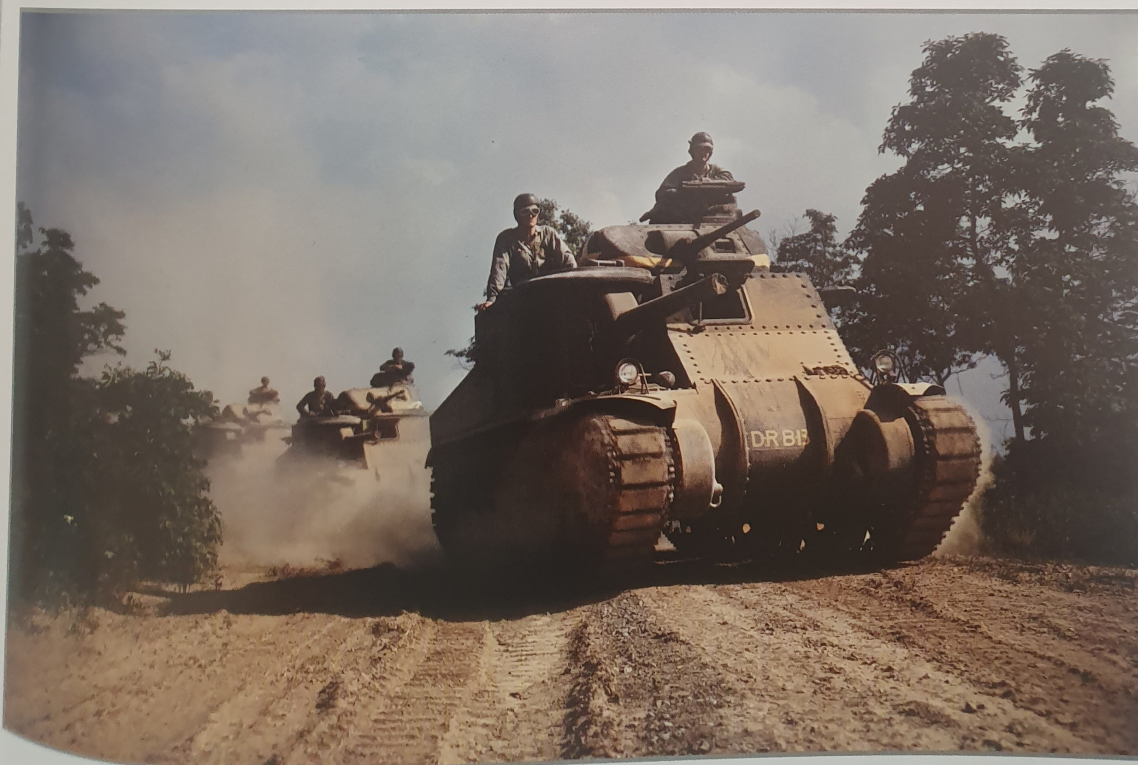
Above: The muzzle covers for the hull-mounted machine guns can be clearly seen in this view of another M3 advancing along a dusty Fort Knox tank trail in June 1942. Unfortunately, no registration numbers are visible to aid in identifying when the tank was built or by whom. Library of Congress
