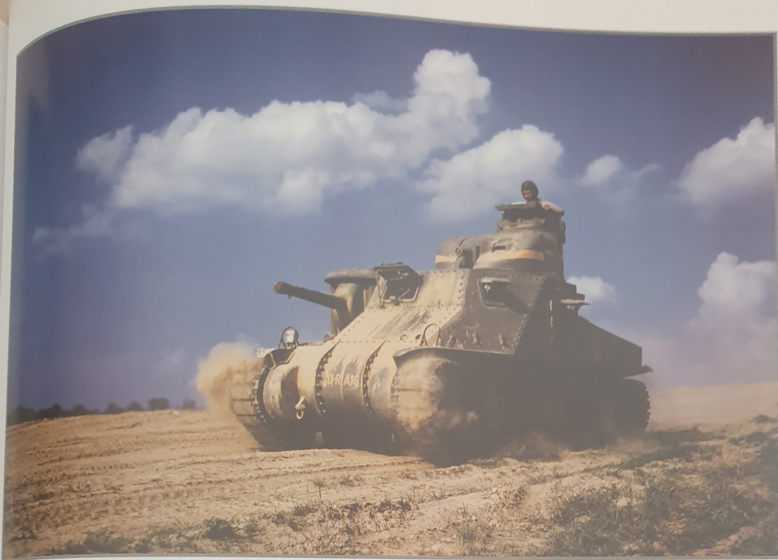
Above: Also seen at Fort Knox, Kentucky, during June 1942, this M3 was possibly completed during the late 1941–early 1942 37mm gun shortage. Within the yellow star on the turret has been stenciled in “AFS,” for Armored Force School, in black. Library of Congress
