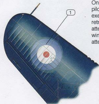
Upper wing roundel position for the all-over Glossy Sea Blue NZ5617. The aircraft had 48 inch roundels above and below both wings.
