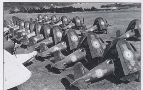
FG-1Ds at Hobsonville airfield ready for barging to the Auckland wharves and loading onto HMS Glory for their trip to Japan. Note the rough over-painting of the older 'operational' roundels. (via P. Mossong)
