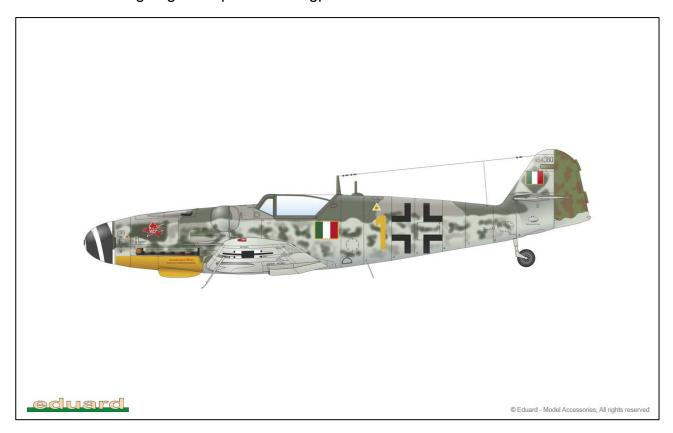
**D: Black 8** – Oberleutnant Rolf Schlegel, CO of 10/Jg4, Juterborg-Damm, Germany, March 1945.Rlm76 over RLM 76 with Black/White/Black RVD bands on the rear fuselage. This machine shows evidence of repainting from an earlier scheme as the number has been applied over a large patch of RLM74. It carries a 300 litre drop tank and rack.
