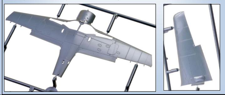
To the lower wing section is added a wing spar, some structural detail in a choice PE or styrene, some piping, the inboard MG151 cannons, and the wheel well roof. The underside exhausts stubs are provided as an insert in the bottom cowl panel molded with the lower wing, with a separate pipe run for cylinder #8 to fit and exit through its own hole in the panel. The separate ailerons can be attached once the upper wing surfaces are in place.
