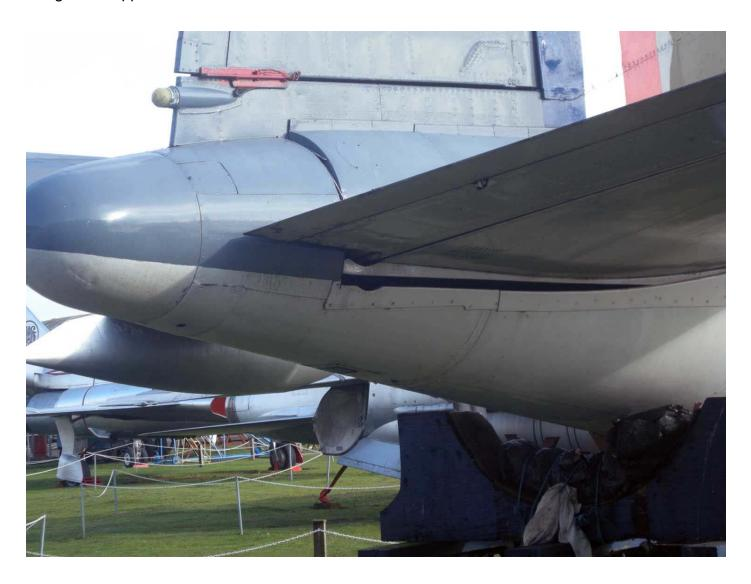
From this, one can note the arrangement of the moving tailplane, and the section of the upper rear fuselage that moves with it.
