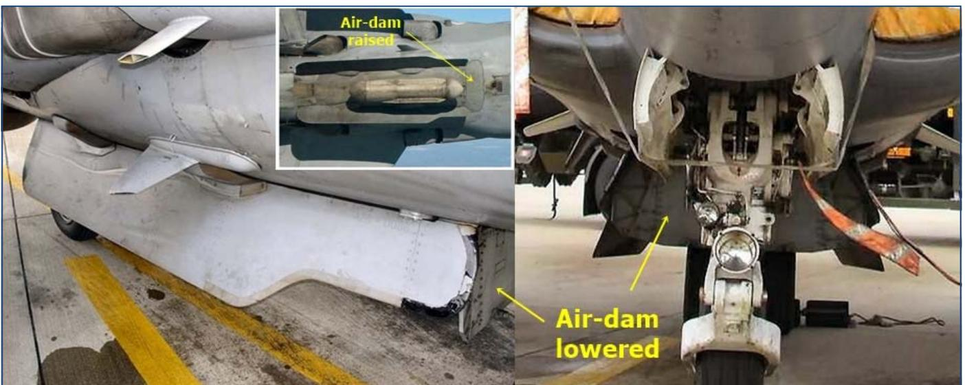
The kit includes the engraved outline of the air-dam, but it will take a bit of effort to replicate a lowered dam and its housing that is really required by a model on its undercarriage (the kit does not provide an in-flight undercarriage option).
