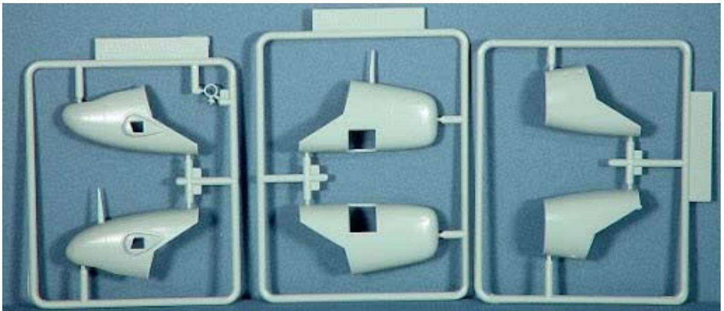
On the left is the standard canopy parts sprue, on the right is the clear nose for the “Droopsnoot” Option.
